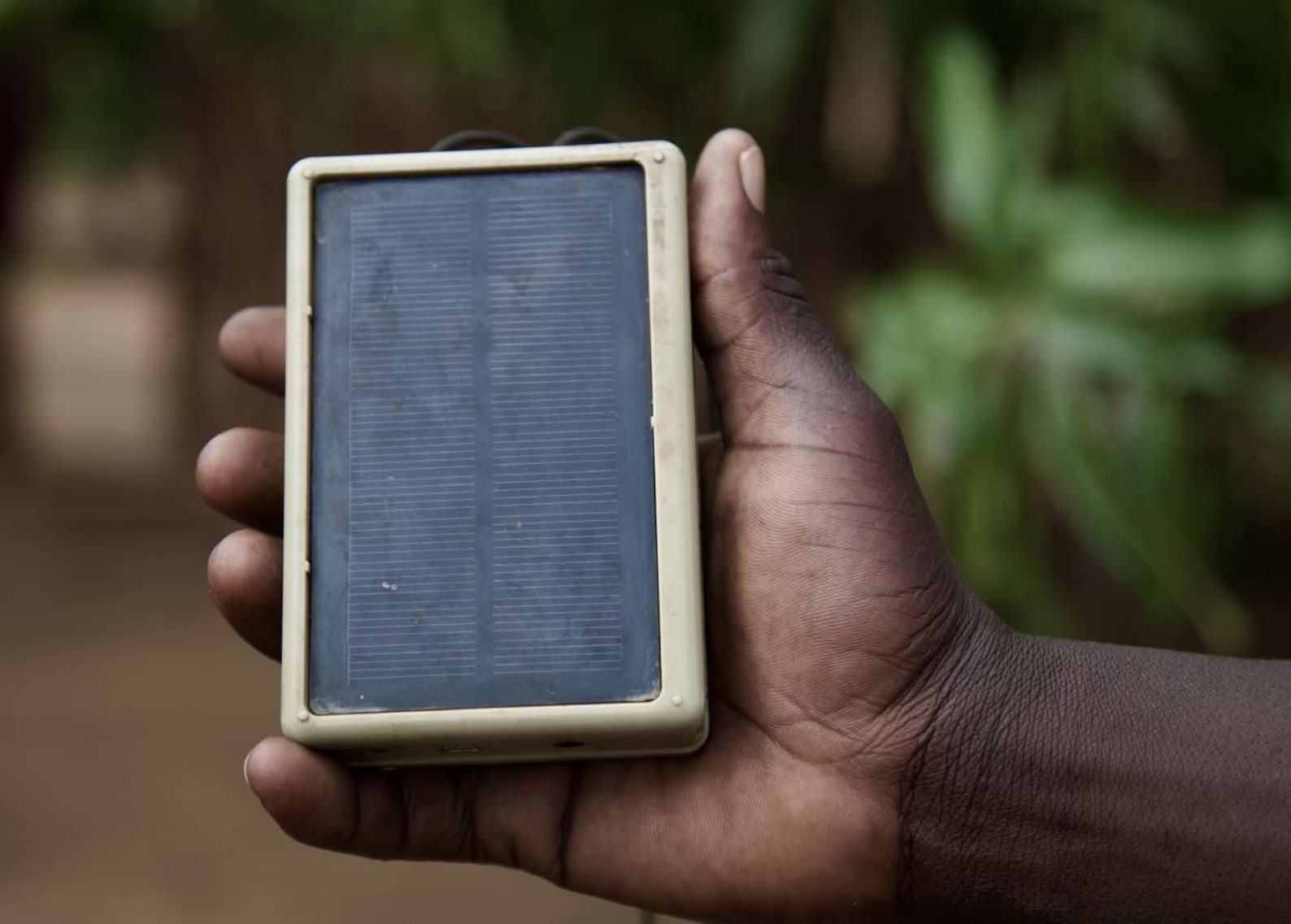
© U-Learn. Solar powered portable wireless radio in Palabek Refugee Settlement
