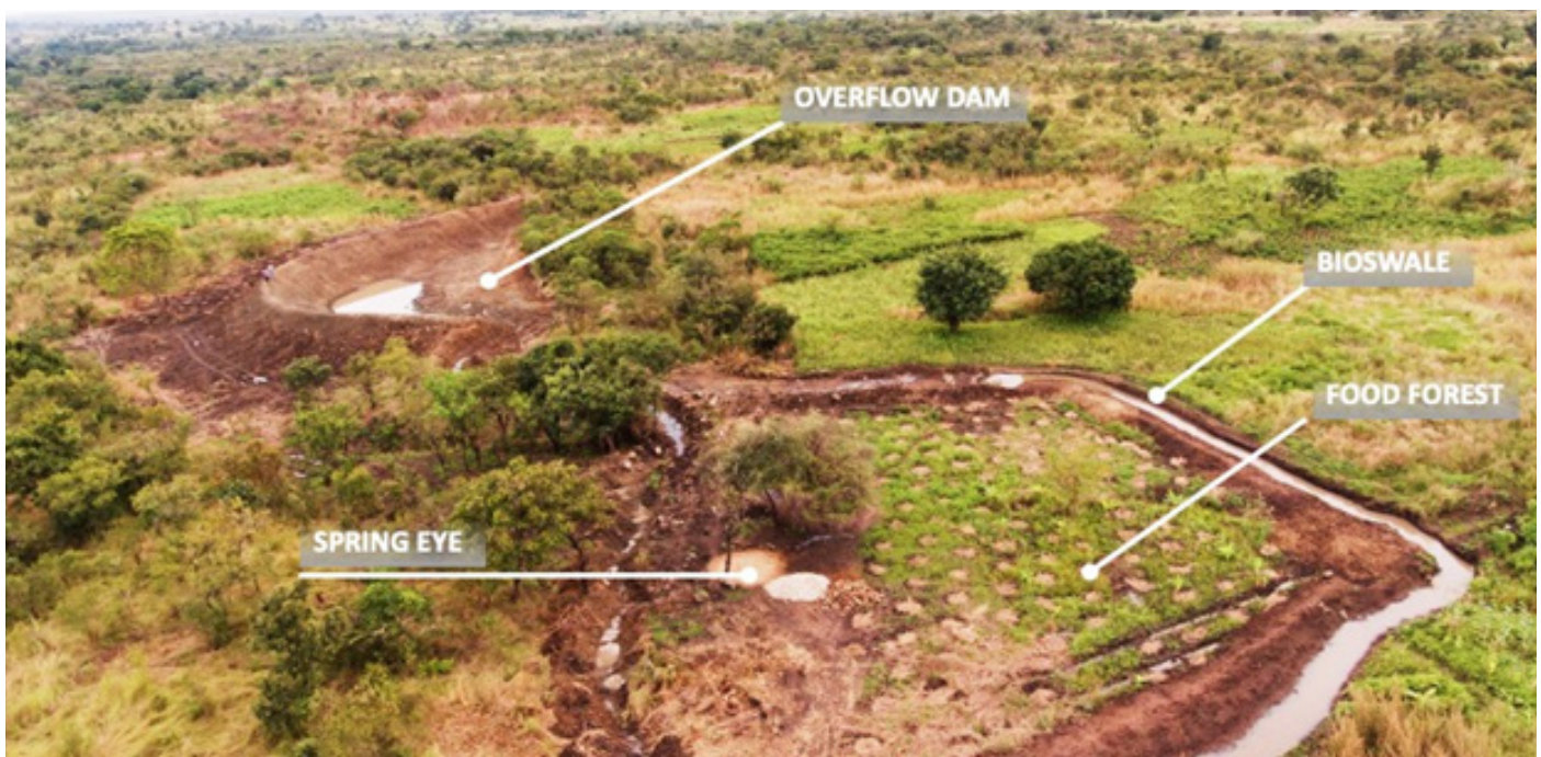
Spring/Ground Water Recharge – Water Management a round a spring source – Pakele Sub-County, Adjumani District, Uganda
